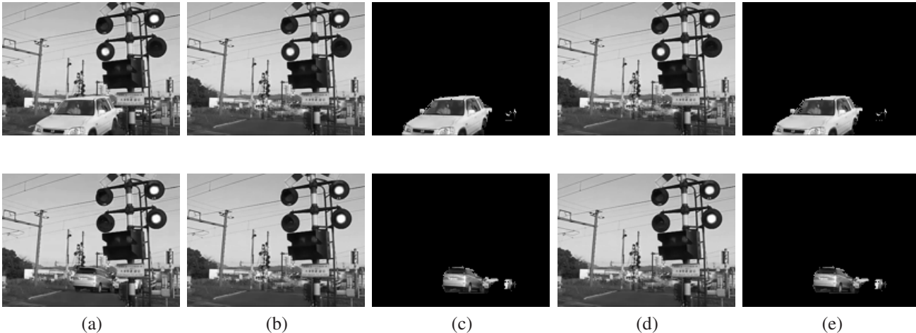
Figure 9. Two traffic light statuses. (a) input frames; (b) subtracted background with batch dictionary update; (c) foreground in batch mode; (d) background with online dictionary update; (e) foreground by our online algorithm.
